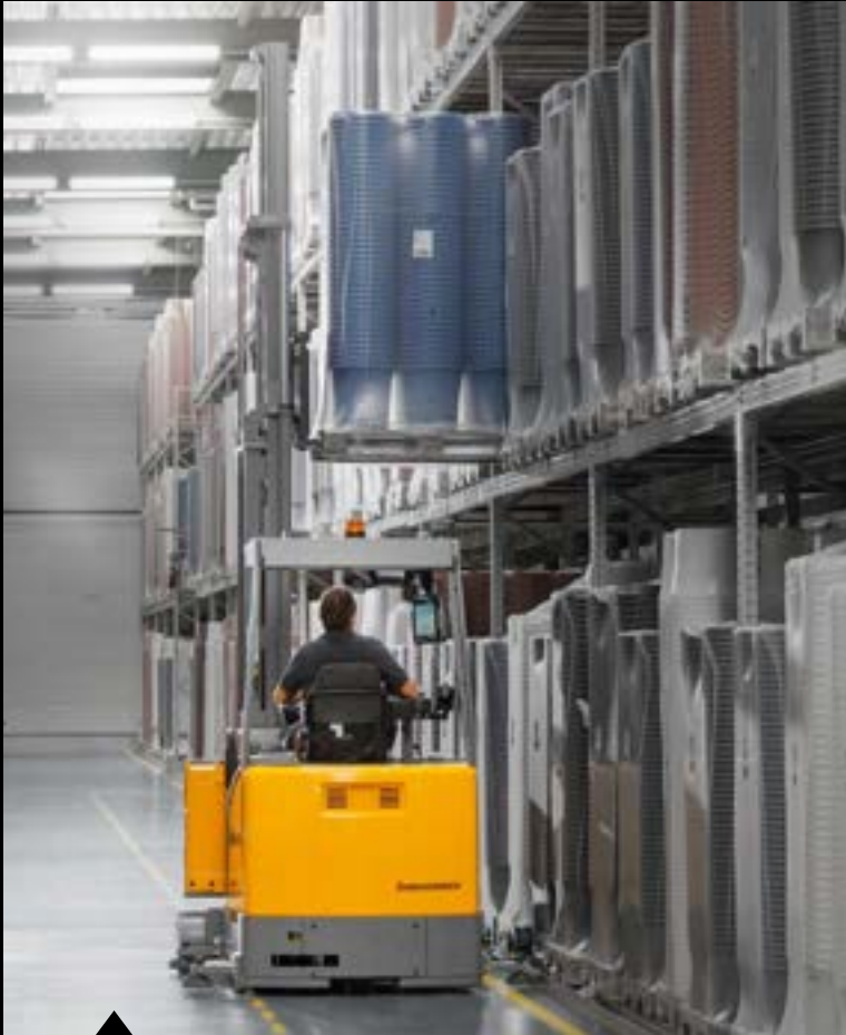
The truck is based on the man-down principle, whereby the fork goes up and the travel platform remains on the ground.
