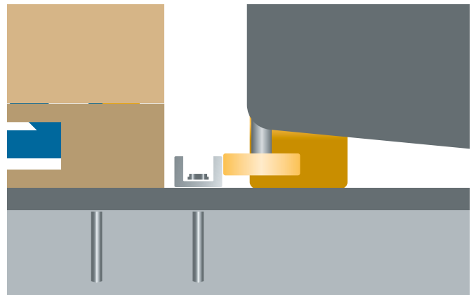
Fig. 6 Low guide rail, e.g. U profile 65/42/6.
