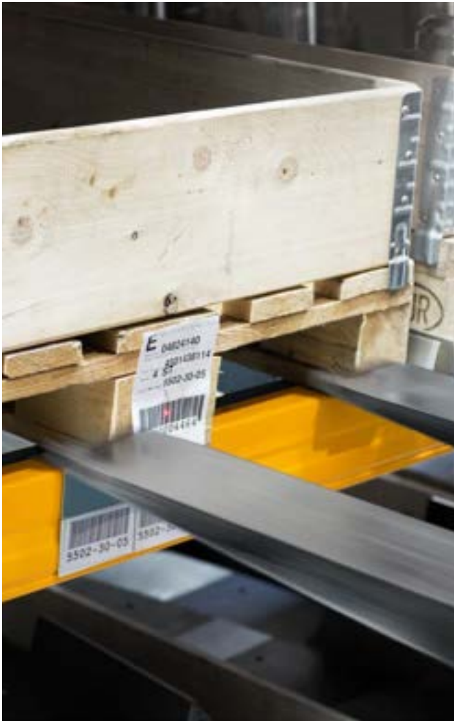
Automatic scan carried out by fork carrier.
