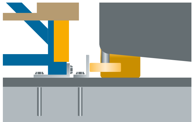
Fig. 5 High guide rail, not cast, e.g. L profile 100/65/11.
