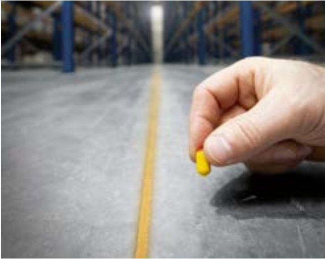
End of aisle control by transponder.
