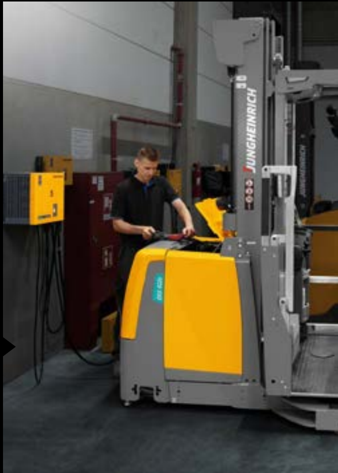
Simple charging of Li-ion trucks.
