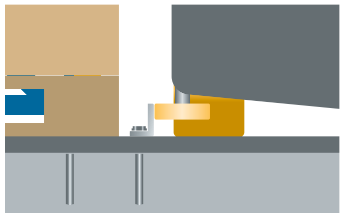
Fig. 7 Low guide rail, e.g. L profile 40/60/8.
