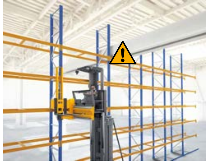
Travel/lift cut-outs in front of an obstacle (intersecting aisle).
