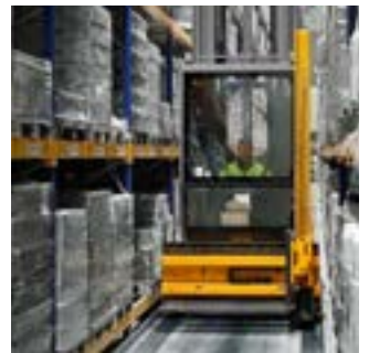
In the heated cabin, operators are safely protected from the cold ambient temperature.
